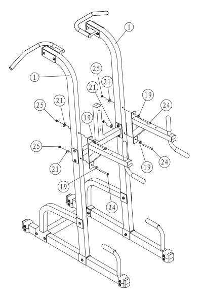
**STEP 3** Connect Elbow Pad Support Frame (4) to Upright Frame (1) using Bolts (24), Washers (19), Large Washers (21) and Nylon Lock Nuts (25).
