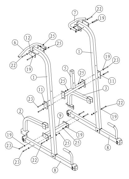
**STEP 2** Connect Back Pad Support Frame (5) to both Upright Frames (1) using Bolts (23), Washers (19), Nylon Lock Nuts (25) and Small Plates (11). **NOTE:** Small Plates (11) are to be placed on the outside of the machine.
