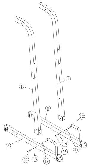
**STEP 1** Connect Upright Frame (1) to Base Frame (8) using Bolt (22), Washers (19) and Nylon Lock Nut (25).
