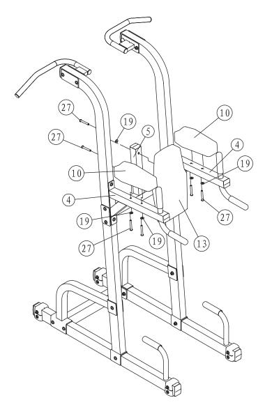
**NOTE:** Hand tighten bolts and nylon nuts until machine is fully assembled.
